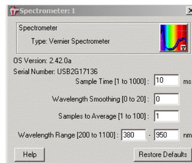
usable spectrum is produced. Changing the Wavelength Smoothing to “0” and Samples to Average to “1” will speed up the data collection.
